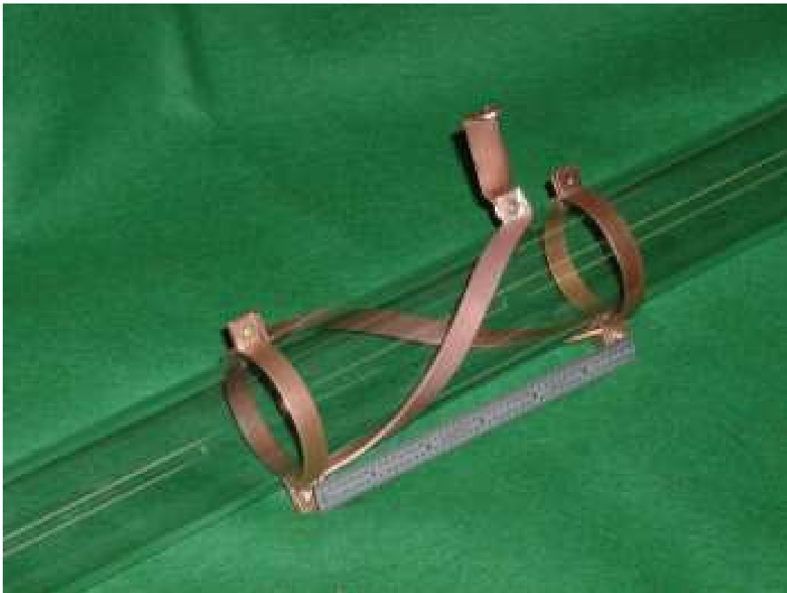
Figure 3.2: Photo of a right-helical antenna mounted on the Mini-RFTF.
